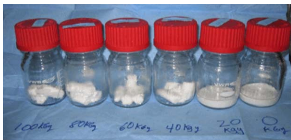
Figure 13. Electron beam crosslinked hydrogel formulations with radiation dosages ranging from 0 to 100 kGy (right to left) showing how electron beam dosages above 20 kGy lead to non-injectable hydrogels. [Color figure can be viewed in the online issue, which is available at wileyonlinelibrary.com .]
